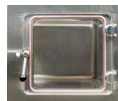
Integrated transfer chamber w/ radius ball corners for optimal cleaning
