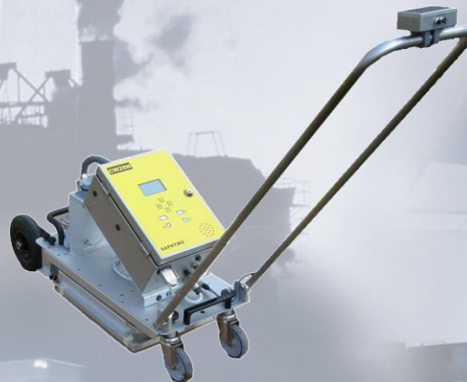
\alpha and \beta floor contamination monitor CW 28-N
